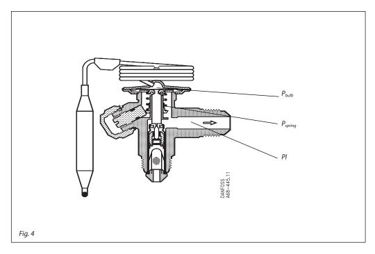
The valve function is controlled by the intermediate pressure (PI) acting under the diaphragm and the bulb pressure derived from the discharge gas temperature across the diaphragm (fig. 4).
