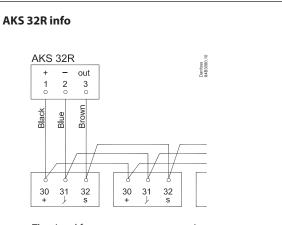
The signal from one pressure transmitter can be received by up to ten controllers. There cannot be a significant drop in pressure between the pressure transmitter's position in the suction line and the S2 temperature in the individual evaporators.
