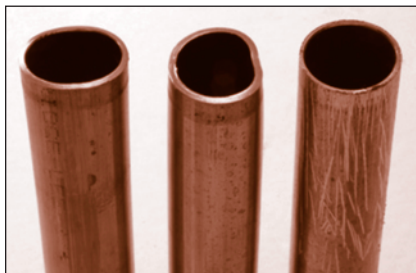
FIGURE 45: Inspect tube for imperfections
