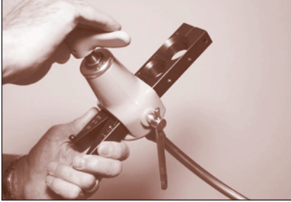
FIGURE 31: Lowering the flaring cone into the tube end
