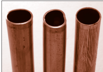
FIGURE 33: Inspect tube for imperfections
