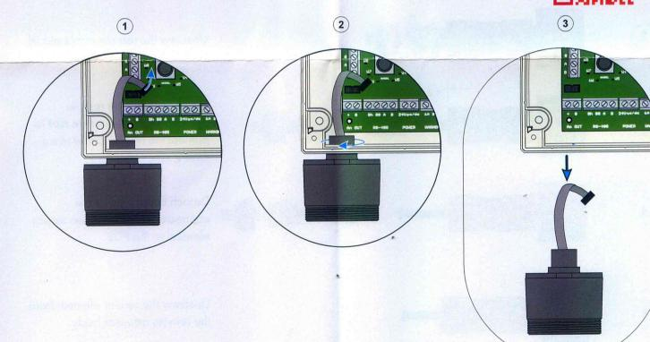
Detach the ribbon cable connector connecting the sensor element to the main PCB.
