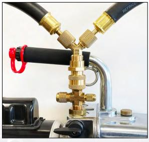
Increase speed of evacuation with the Dual Y Coupler Connector and two large diameter hoses.
