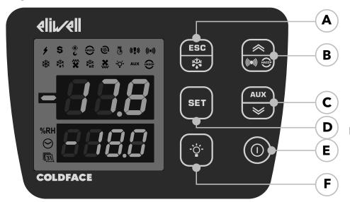
**RCN**••••••• models: when the HACCP Module is connected and the Bluetooth connection to the Eliwell Air App is active, the btL label appears on the TOP DISPLAY and the BOTTOM DISPLAY and icons are turned off.
