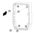
4) Fit the hinges to secure the cover.
